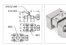
\* Reverse the jaws to switch from ØD1 to ØD2 Includes a #10-32 M/M stud with jam nuts
