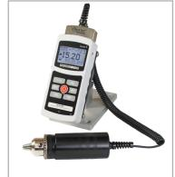
M5I is shown mounted to an optional AC1008 tabletop stand with Series R50 torque sensor
