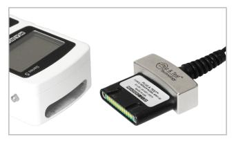
^ Unique Plug & Test® technology allows for interchangeable sensors to be used with a Mark-10 model M7I, M5I, or M3I indicator. All calibration and configuration data is saved in the smart connector.
