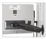
Test frame part numbers ending in "-IMT", for example Model F305-IMT, include a Windows tablet with attached ball mount and mounting bracket, packaged separately. The mounting arm is pre-installed into the front right slot in the test frame column via two screws.
