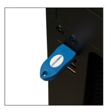
The dongle contains a one-seat license. It must be plugged in at all times to run IntelliMESUR. To run IntelliMESUR on a different device, install the application, then move the dongle to that device.
