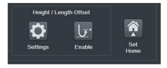
Selecting this button establishes the current crosshead position as **Home**. Refer to subsequent sections for more details on how this position relates to test configurations.
