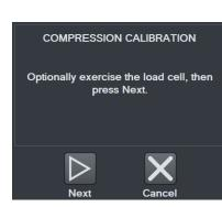
Optionally load and unload the force sensor to full scale several times, then select Next.
