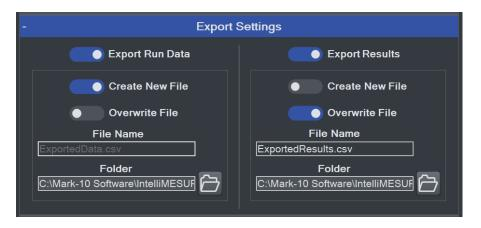
IntelliMESUR<sup>®</sup> can automatically export data from a single run or results from a batch of runs, or both. Files are exported as .csv using the same formatting described in the manual export function in the **Running a Test** section.
