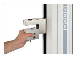
While holding the force sensor in place with one hand, use an Allen wrench with the other hand to tighten the screw that joins the force sensor to the crosshead, as shown below:
