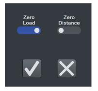
A Zero step zeroes the load and/or distance. Make the desired selections.
