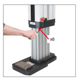
4. Position the test frame vertically and reinstall the sheet metal covers, as shown below:
