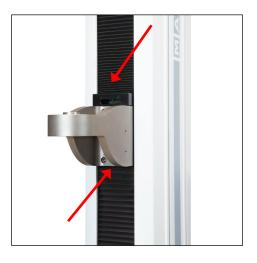
**2.** Using a brush, apply a small amount of general-purpose bearing grease to the screw, as shown in the image below:
