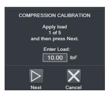
Apply the indicated compression load using the **crosshead motion controls**. The load value defaults to even intervals. For example, for a 50 lbF force sensor with 5 calibration points, the first default load value is 10 lbF. All load values may be edited by up to  $\pm 20\%$ .
