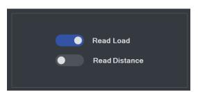
A **Data** step saves the current load and/or distance value in the **Results** table. Make the desired selections.
