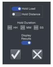
Hold a load (as described in **Basic Test** setup) or hold a position. Specify the hold period in hours, minutes, and seconds.
