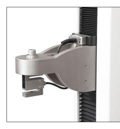
Grips and fixtures may be threaded onto the underside of the sensor.
