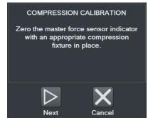
Zero the indicator associated with the master load cell. Engage the calibration fixtures, and ensure that there is no load applied to the force sensor. Then select **Next**.
