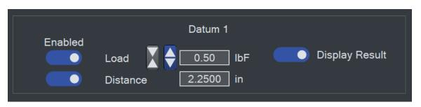
A datum establishes a local offset of load and/or distance. When the datum step is reached, the load and/or distance will change by the values set in the **Load** and **Distance** fields. Enable one or both of these fields.
