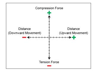
The most common method to plot a curve is to plot up and to the right. To achieve this trajectory, or other type of trajectory, data for each axis may be inverted to compensate for the plotting protocol mentioned above.
